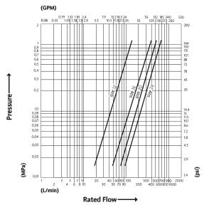
Test performed according to ISO 18869
